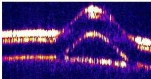
Picture below: Seam defect. The upper film separates from the substrate.
