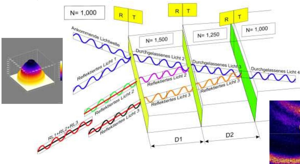
In the graphic, R stands for reflection and T for transmission. N denotes the refractive index of the material and D denotes the layer thickness.
