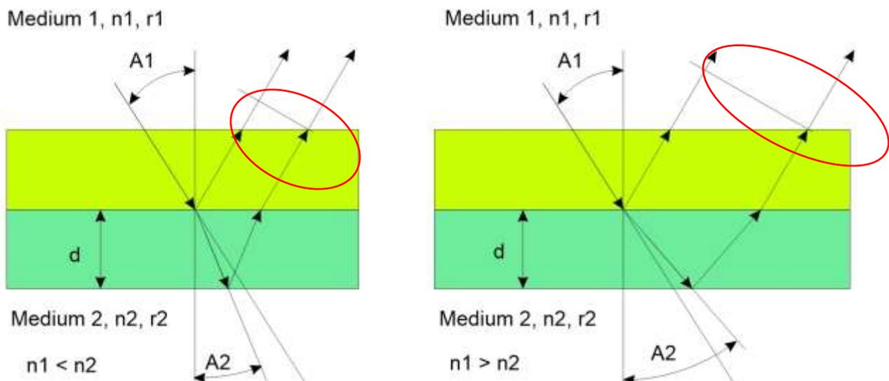
The retardation is, in contrast to reflection, a periodically variable size and clearly a function of the thickness of a layer.
