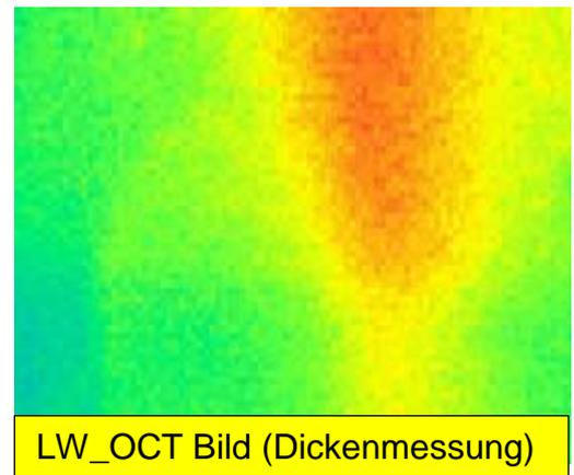
When using radar sensors in driver assistance systems, electrically active layers have an effect on the accuracy of the measured signal, which is why a homogeneous and defined layer thickness is of interest for vehicle coating.
