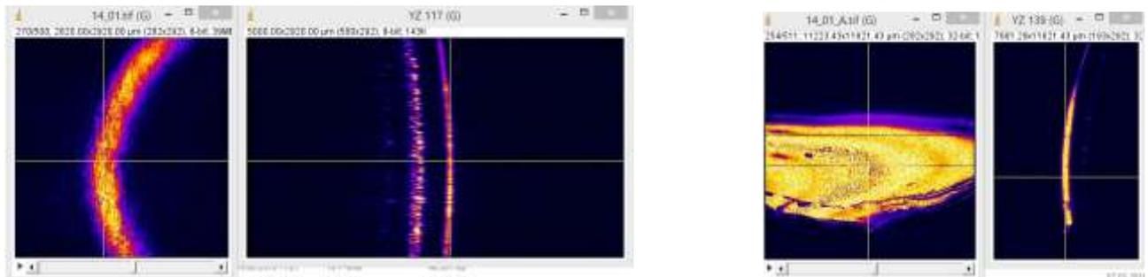
Each single image from the stack can be consulted for evaluation. The distance from image to image can be selected between  $<1 \mu\text{m}$  to higher than 1 mm. In the OCT method, the z-axis is decoupled from the lateral resolution, in contrast to conventional imaging or confocative methods.
