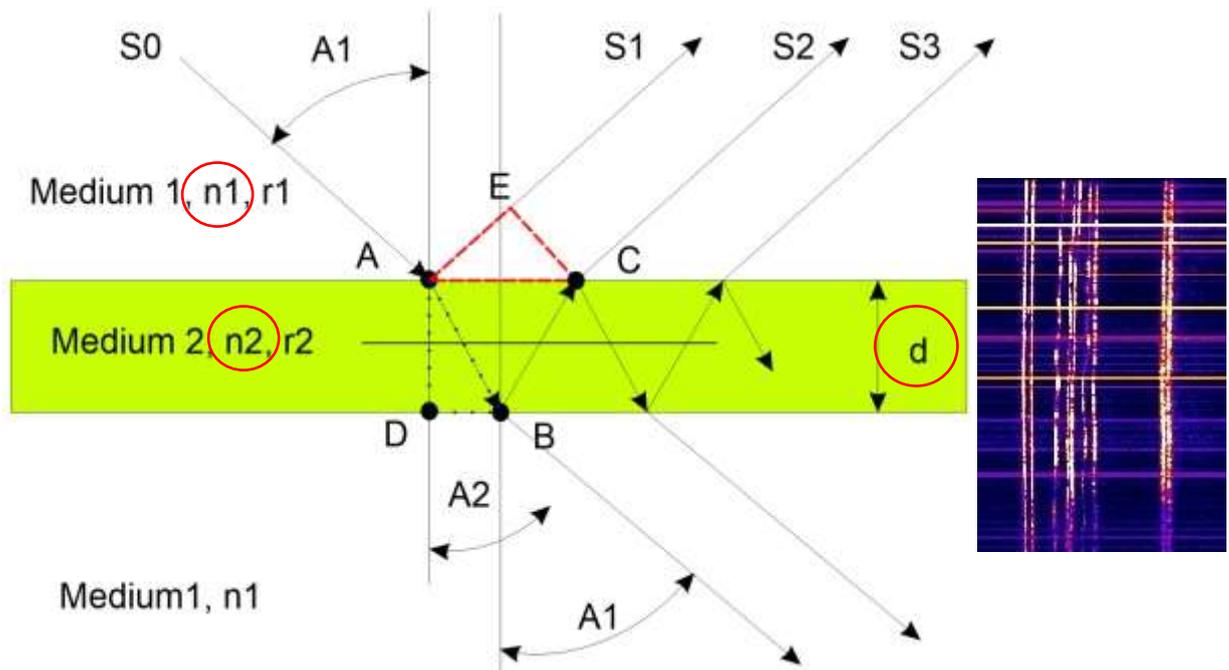
In fact, it is relatively easy to detect the spatial position of the surface of an object and to measure the thicknesses of the individual layers from the path difference (graphic above, distance CE), provided the refractive indices are known. If the refractive indices are not known, two monochrome light sources are used to extract the desired layer thickness from the signals. The following graph shows the same layer thicknesses but unequal refractive indices. The gait difference is very clear.
