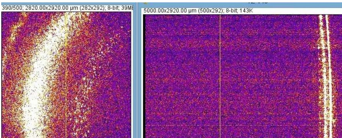
With a single light pulse, all interfaces between individual films or bearings of a coating appear because there is a difference in refractive index.
