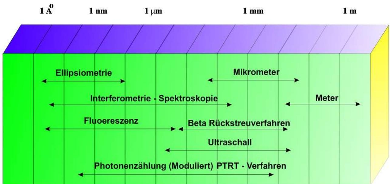
Overview of methods and methods for the measurement of all kinds of coating thickness.
