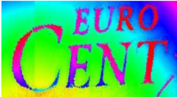
The measured levels of each pixel yield the exact three-dimensional reconstruction of the surface. Due to the intensity information to obtain a high-resolution deep sharp image. With optional use of a color camera, a color image of the surface can be produced in addition.
