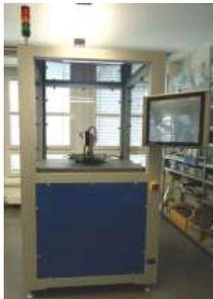
With two probes, the volume, all dimensions, thickness, weights, profiles, markings, flatness of surfaces or their parallelism and planarity can be measured in one step, accurately and quickly.
